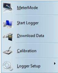
Click on **Download Data** in order to transmit the saved measurement data to the computer. Measured data will be output in a **\*.bin** file and afterwards converted into an **ASCII** file. The **\*.bin** file is compressed and can be archived. The **ASCII** data are required for charting with the InfraLog Graph-Tool (only for Light/Enhanced versions) and for import into third party applications.
