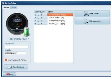
The available sensor inputs/slots are depicted on the logger image on the left. In addition you can see the battery status. If the battery is green it is still in good shape and you can use the logger. A red battery indicates that the batteries should be replaced soon. In this case you should only make very short measurements
