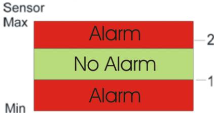
Two alarm areas are active on selected channel. If sensor reading is higher than (Threshold1 ± Hysteresis) and lower than (Threshold2 ± Hysteresis) the alarm is inactive. Otherwise there is an alarm.
