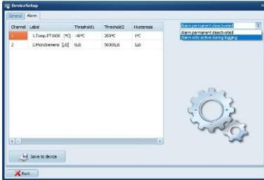
Enable the alarm function by selecting **Alarm only active during logging**. Should you not require an alarm select **Alarm permanent deactivated**.
