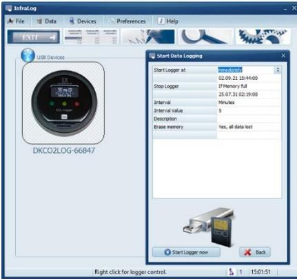
You can configure the following options: **Start Logger at**, **Stop Logger**, **Interval (Unit/Value)**. In addition, you can specify the measurement site by giving a **Description**.
