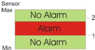
Only one alarm area active on selected channel. If sensor reading is higher than (Threshold1 ± Hysteresis) and lower than (Threshold2 ± Hysteresis) the alarm is active. Otherwise there is no alarm.
